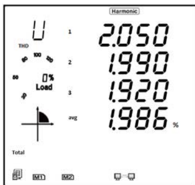
Figure 3-25 Harmonic Distortion Reading
