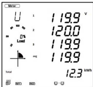
Figure 3-3 Three-Phase Voltage Page
